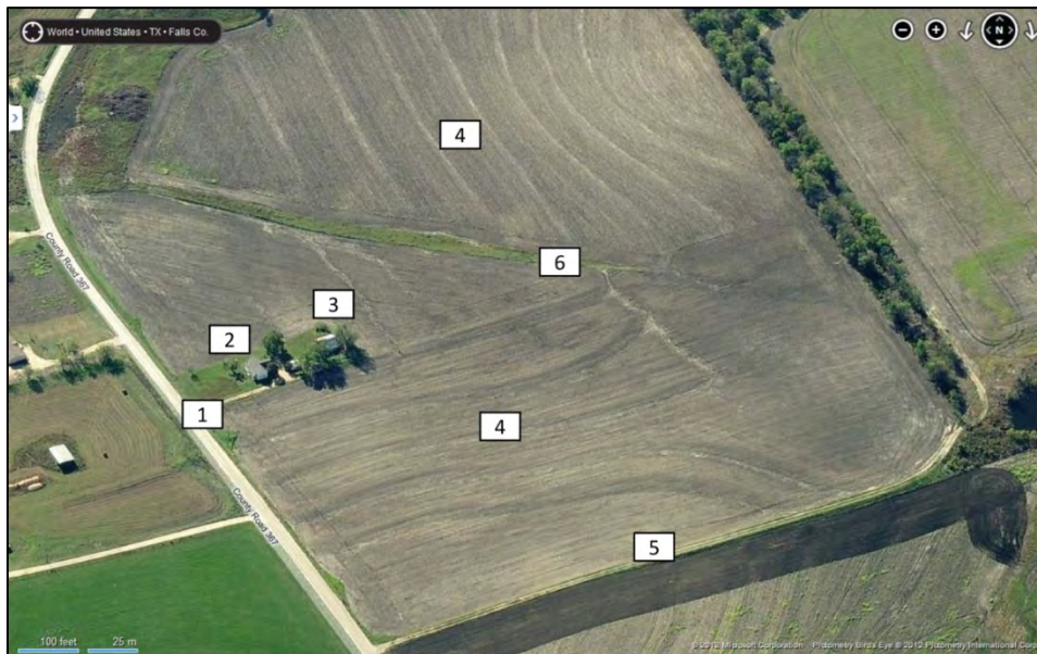
Figure 3-17. Aerial View of Farm on CR 367 in Falls County, 2012. This image illustrates a farm with landscape features (a drainage ditch that bisects the property and contoured fields) that help indicate that this is a property that focuses on cultivation. The numbers on this figure correspond to the specific features on the property: 1. Main entry driveway that provides access from the public road to the domestic work zone; 2. Domestic work zone; 3. Agricultural work zone; 4. Fields that have been contoured to allow for water movement into the drainage ditch; 5. Driveway on the southeast side of the property that provides access to the fields; 6. Drainage ditch that runs through the center of the fields. Source: Bing Maps.
