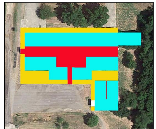
Figure 9. A conceptual design plan identifies space for apartments in the building (shown in blue). Red is common space and yellow could provide gallery/exhibit space.
