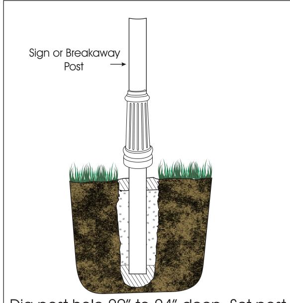
Dig post hole 20" to 24" deep. Set post in hole, add 40 pounds of concrete. Check for levelness & tamp concrete. Fill hole with dirt until level with ground.
