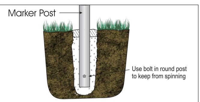
Dig post hole 24" to 30" deep. Set post in hole, add 80 pounds of ready-mix concrete. Check for levelness & tamp concrete. Fill hole with dirt until level with ground.
