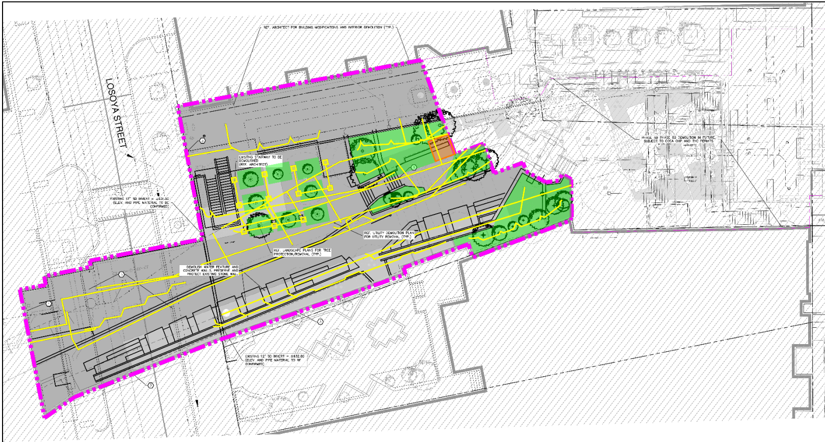
Figure 17. Architectural drawing of proposed demolition activities in Project Area. Trees highlighted in green, utility lines highlighted in yellow, and the elevator pit highlighted in orange. Concrete walls are designated by the black sketch lines.
