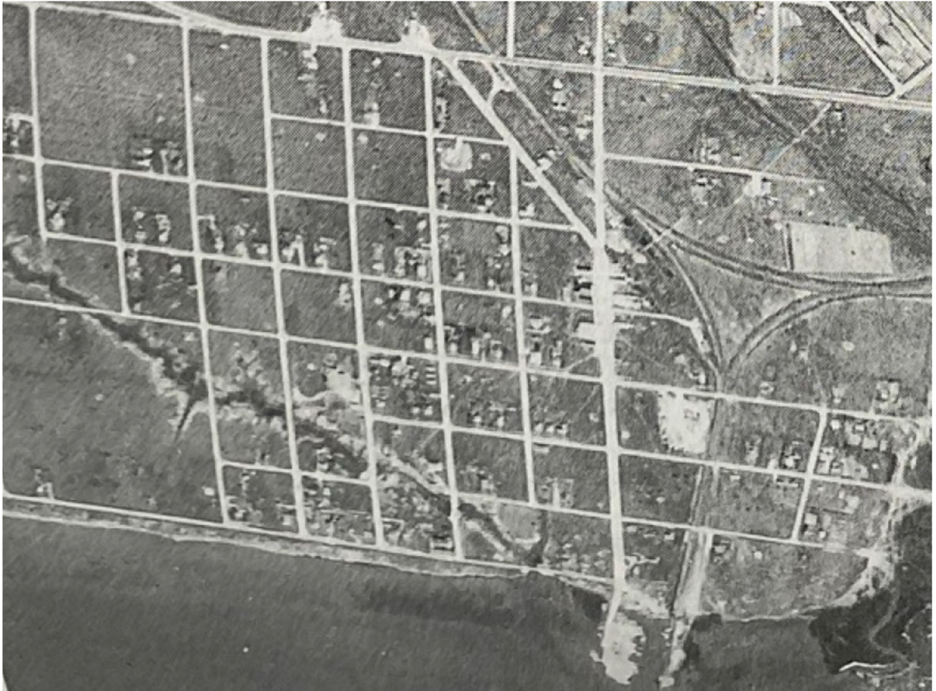
Figure 21. This undated aerial view of Seadrift shows several homes built along the town's platted square blocks. A small cluster of downtown buildings is west (left) of the railroad's triangular wye (Johnstone 2003b, 4:2).
