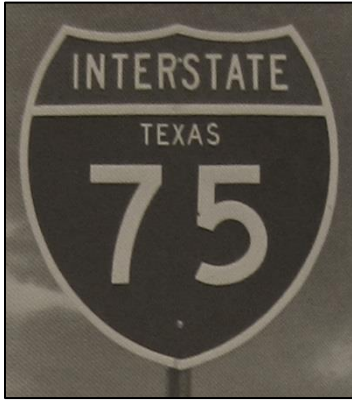
Figure 119. Example of the new, uniform markers developed for the Interstate Highway System. The design of the new interstate highway sign introduced a new but soon-to-be familiar feature of the American roadside landscape. Unlike the U.S. highway signs that were black and white, new interstate signage used red, white, and blue. A white border outlined the distinctive shape and divided the top/crown from the main body. The crown had a red fill with the word “INTERSTATE” in white letters. The main body of the shield was blue and identified the state and interstate highway number, again in white. Although this image is from the Texas Department of Transportation, this highway designation was not adopted or used in Texas and is only an illustration of what was being considered during the initial development of the Interstate Highway System in Texas. Source: Texas Department of Transportation, Communications Division, Media Production, Photo Library, Austin, Texas.
